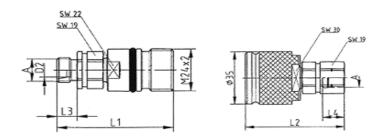
Screw type couplings of the HS series are coupled by simply screwing the carrier and probe halves together until the thread contacts the limit stop.
