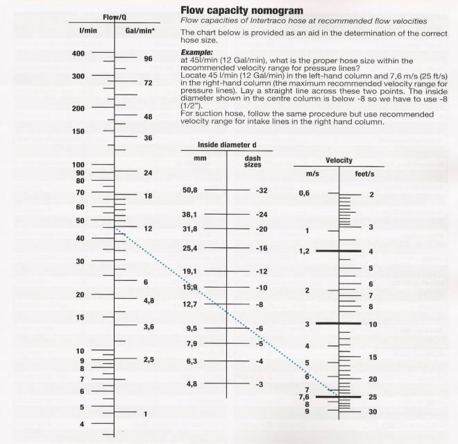
$\mathbf{Q}$  = flow in liter per minute or US Gallons per minute  $\mathbf{V}$  = velocity in meter per seconds or feet per seconds  $\mathbf{d}$  = hose inside diameter (mm /dash size)
